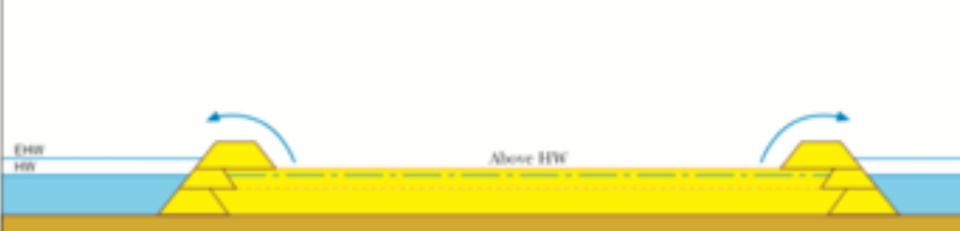
IL.C.3 LANDFILL 1: WATER MANAGEMENT BY GRAVITY DRAINAGE & PUMPING (AT EHW)
