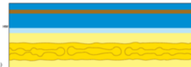
I.B.2 Submerged Offshore Breakwater - Reef Type (Sand Retaining Dam, Wave Energy Reduction)
