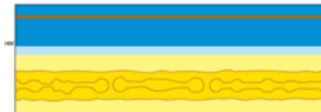
I.B.1 Submerged Parallel Berm / Perched Beach (Sand Retaining Dam)
