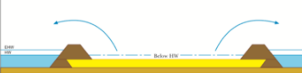
IL.C.2 POLDER 2: WATER MANAGEMENT BY PUMPING IN COMBINATION WITH LANDFILL
