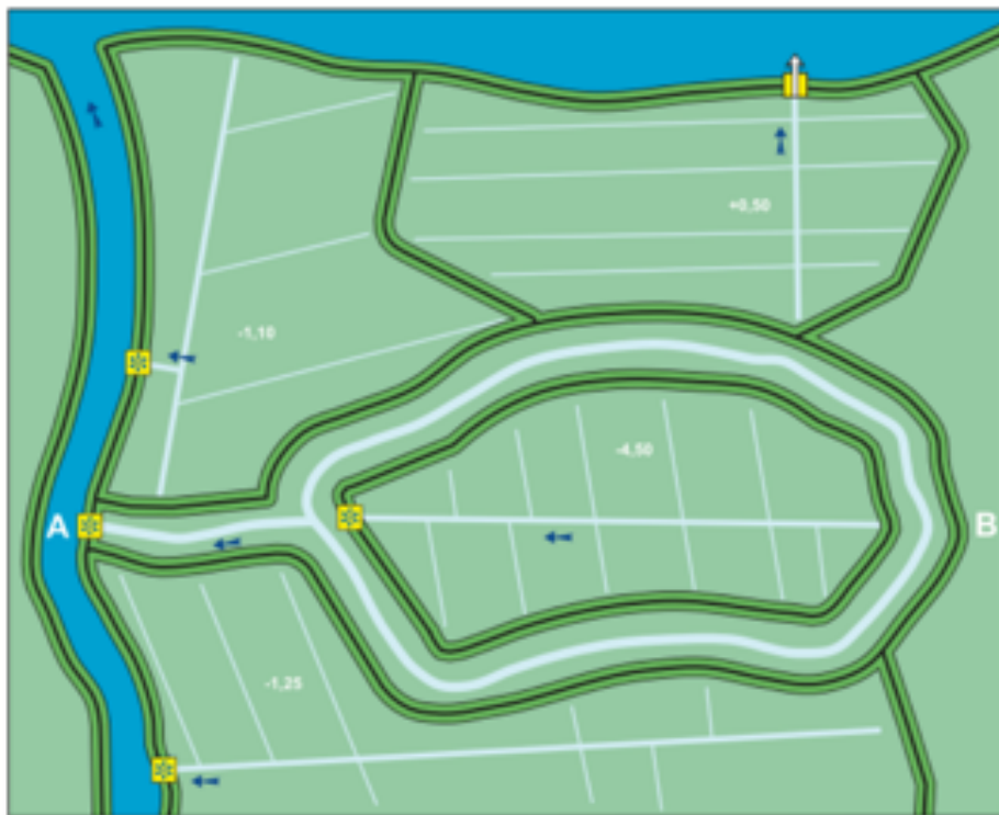
IL.C.2 POLDER 2: WATER MANAGEMENT BY PUMPING IN COMBINATION WITH LANDFILL
