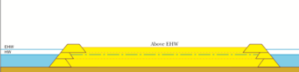
IL.C.4 LANDFILL 2: WATER MANAGEMENT BY GRAVITY DRAINAGE
