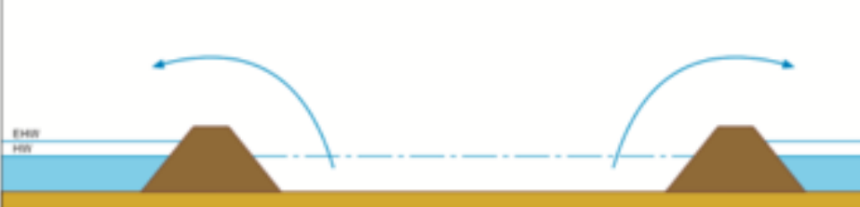
IL.C.1 POLDER 1: WATER MANAGEMENT BY PUMPING
