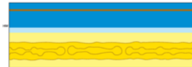
1.B.1 Submerged Parallel Berm / Perched Beach (Sand Retaining Dam)
